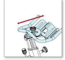
3. Turn pin clockwise to lock. Tighten knob until snug and post is secure without wobble.
