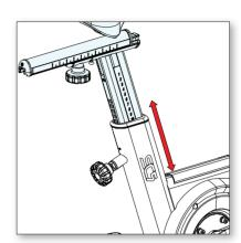
Release pin and turn clockwise to lock. Tighten knob until snug and post is secure without wobble.
